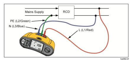
Figure 11. Connection for Test of RCD type B or RCD type A-EV on IT Electrical Systems
