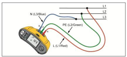
Figure 13. Phase Rotation Test Connection
