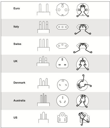
Figure 3. Country-Specific Zero Adapter Configurations
