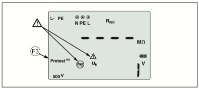
Figure 5. Display for Safety Pretest
