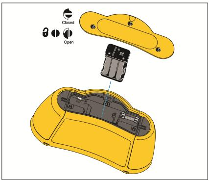
Figure 20. Battery Replacement
