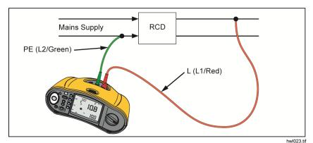
Figure 10. Connection for RCD Test on IT Electrical Systems
