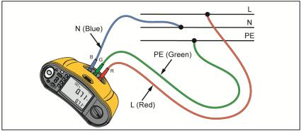
Figure 4. Connection for Safety Pretest
