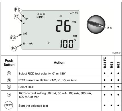
Table 15. RCD Tripping Time Display/Dial and Terminal Settings
