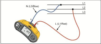
Figure 7. 3-Phase System Measurement
