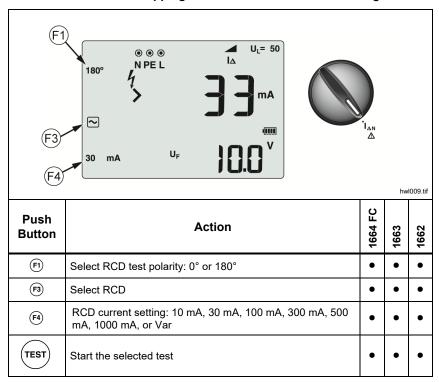
2. Press (a) to select the RCD current rating (10, 30, 100, 300, 500, 1000 mA). If the RCD has a special nominal current setting other than the standard options, you can use a custom setting with the Var mode.
