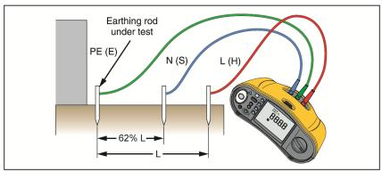
Figure 15. Earth Resistance Test Connection
