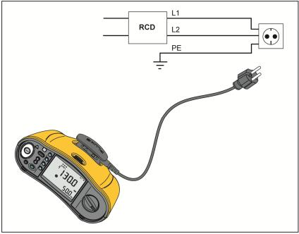
Figure 12. Single Test Lead Configuration
