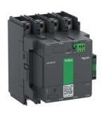
High power contactor, TeSys Giga, 4 pole (4NO), AC-1 <=440V 250A, standard version, 100...250V wide band AC/DC coil
