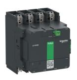
High power contactor, TeSys Giga, 4 pole (4NO), AC-1 <=440V 550A, standard version, 100...250V wide band AC/DC coil
