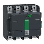
High power contactor, TeSys Giga 630,4P(4NO), AC-1 <=440V 1050A, standard version, 100-250V AC/DC wide band coil
