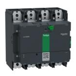
High power contactor, TeSys Giga 800,4P(4NO), AC-1 <=440V 1050A, standard version, 100-250V AC/DC wide band coil
