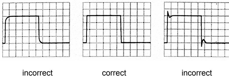
Figure 3-2: Probe compensations
