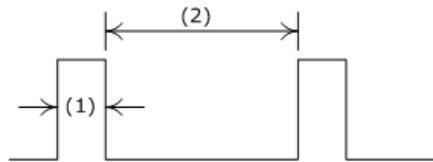
(1): When positive polarity selected, the trigger will take place on the high to low transition of the pulse if the compare condition is match. See figure 5-10.
