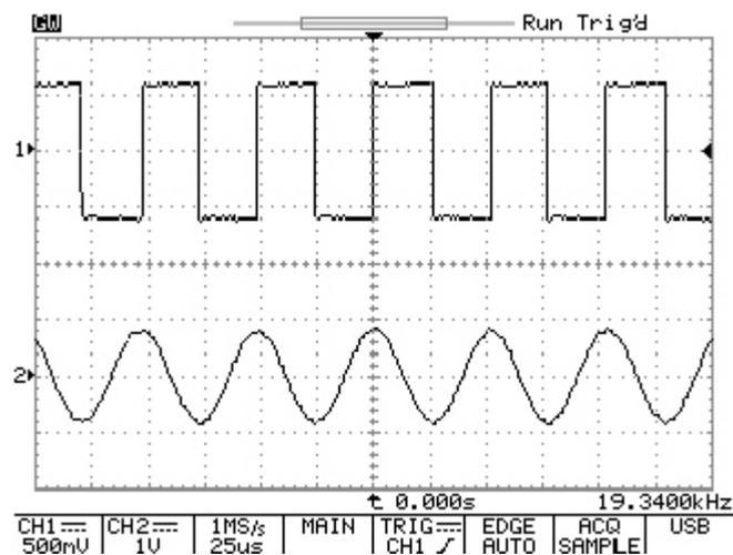
Figure 5-41: A large twelve division waveform display without side menu.
