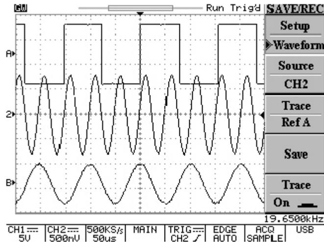
Figure 5-39: Both reference A and reference B are displayed on the waveform area
