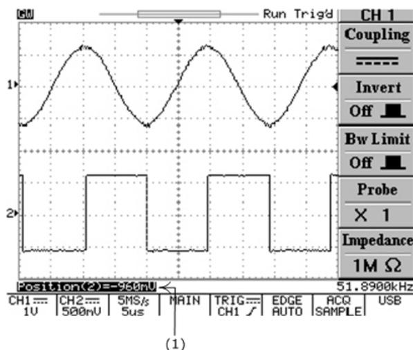
(1): If position of channel1 (or channel2) changed, the vertical position readout will be displayed on here
