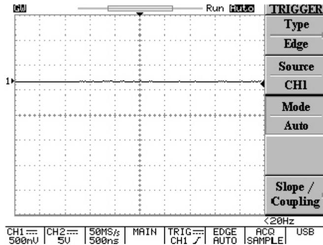
Figure 5-14: The oscilloscope is in auto mode and trigger conditions are not met
