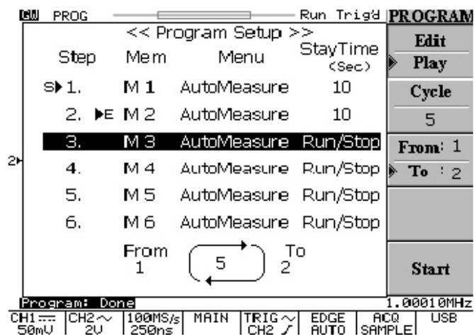
Figure 5-35: the Entire program running is finished
