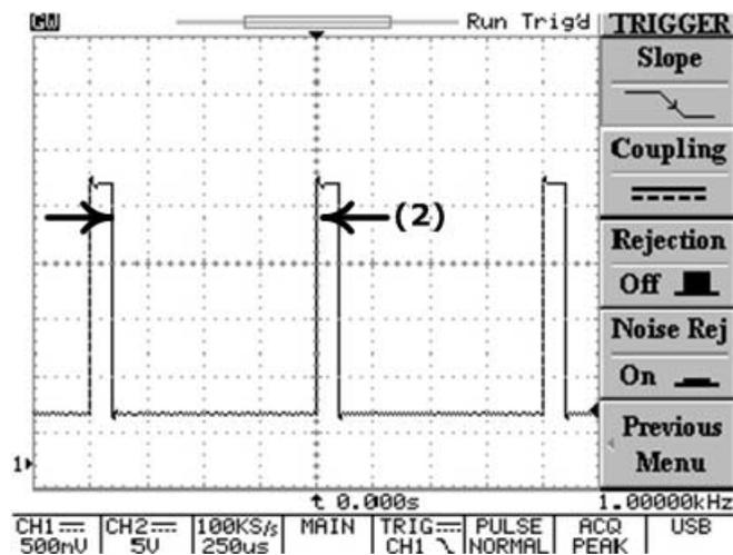
Figure 5-17: Pulse width trigger with negative polarity selected
