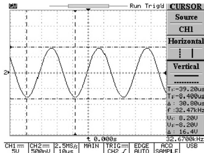
Figure 5-37: Vertical and horizontal cursors measurements
