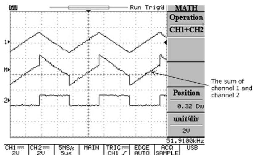
Figure 5-3: Operating the math function (Channel + channel 2)
