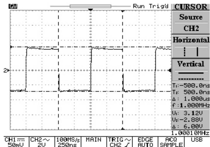
Figure 5-28: Adjusting the horizontal and vertical position for channel two input
