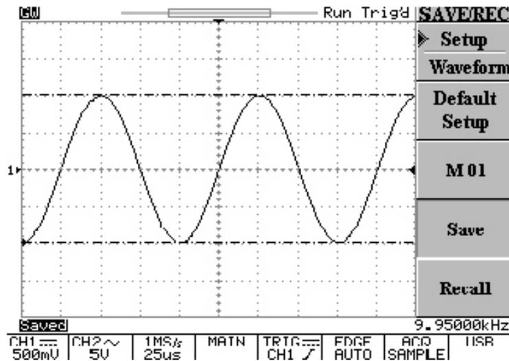
Figure 5-27: Save channel one settings to memory location one (M 01)
