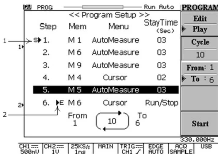
Figure 5-25: Programming for play function of “Program” mode
