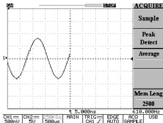
Figure 5-9: Increasing “delay trigger indicator” shifts the waveform to the left
