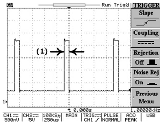
Figure 5-16: Pulse width trigger with positive polarity selected
