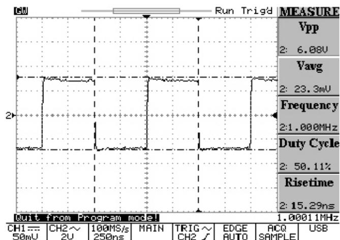
Figure 5-36: Quit the program mode by pressing **AUTO TEST/STOP** button
