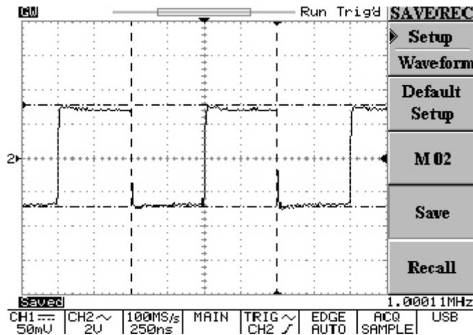
Figure 5-29: Save channel two settings to memory location two (M 02)
