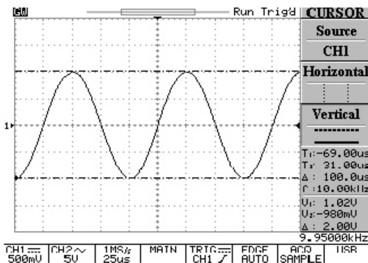
Figure 5-26: Adjusting the vertical position for channel one input of example
