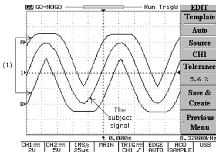
(1): According to the subject signal, the two templates (RefA and RefB) are created by “Template Auto” automatically. The adjustable range (Tolerance) is available from  $\pm 0.4\%$  to  $\pm 40\%$  (or  $\pm 0.04$  division to  $\pm 4$  division).
