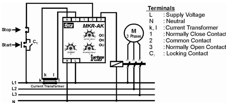
Figure -1 Connection Diagram
